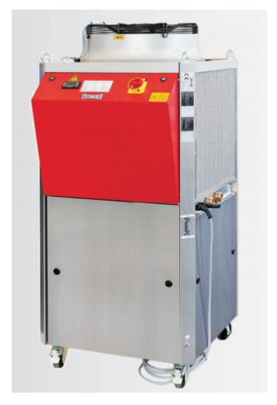
The water chiller MCK consists of a cooling unit in the upper part and a pump plus isolated water tank (made of stainless steel) in the lower section. The unit is conveniently constructed from a frame with removable side panels, allowing easy access to the inner components. The ventilator is assembled at the top part of the unit blowing the warm air upwards.
