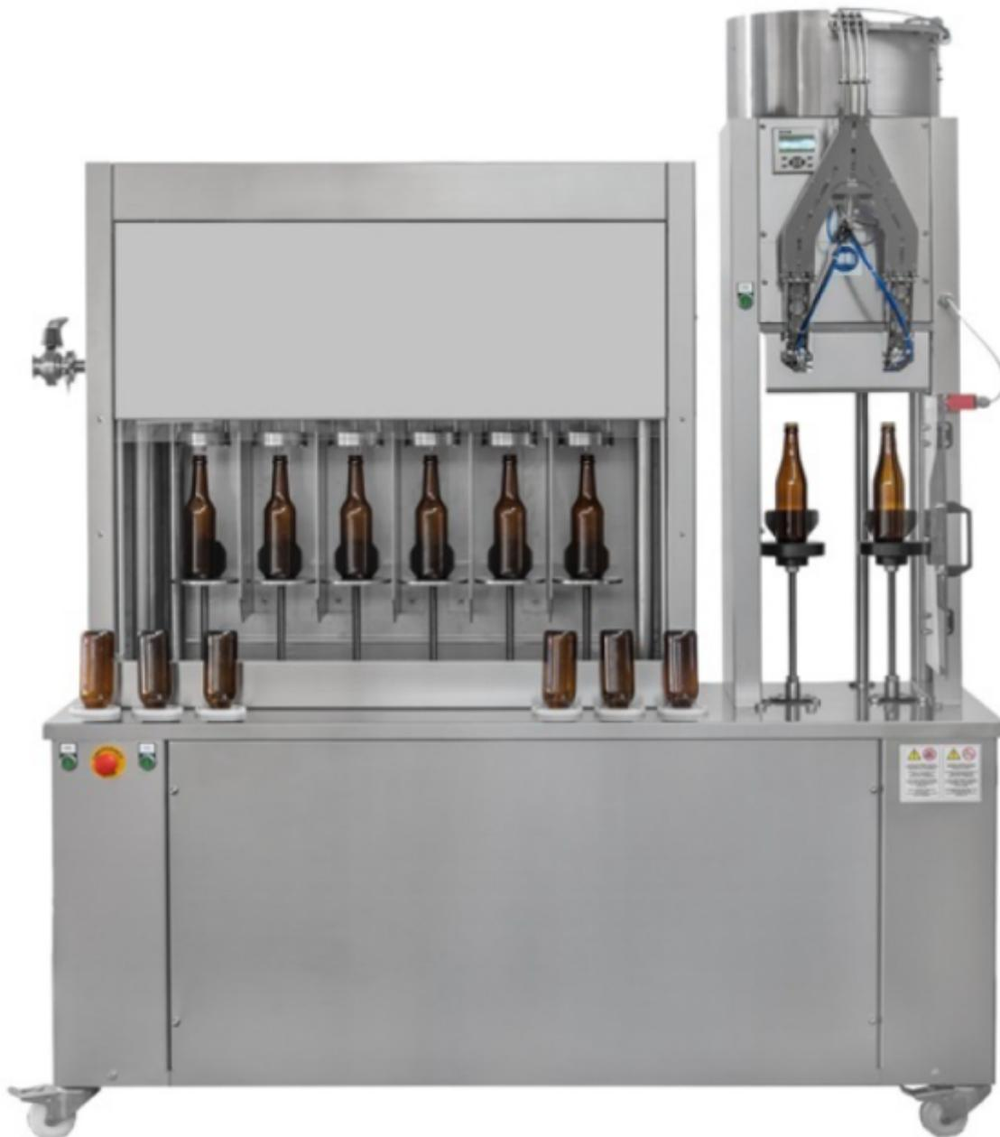
SPARKLING RC 400 Semi-automatic Triblock equipped with a module for rinsing bottles, filling and closing with crown caps.
