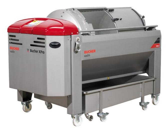
The Bucher XPro is designed to process whole bunches, destemmed and / or crushed grapes as well as fermented pomace. This grape press is especially dedicated for a selection of qualitative batches. Very easy to handle and to use, very compact, the Bucher XPro press fits easily in every winery. Juice bin on wheels with a capacity of 230 liters, DIN DN 40.
