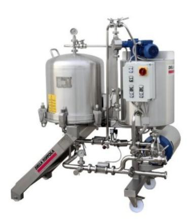
Done correctly, filtering with kieselgur (or micro-filtering) enables a crystal-clear product to be obtained without interfering with its organoleptic qualities, and avoiding the need to perform thermal treatments or sterile filtering processes.
