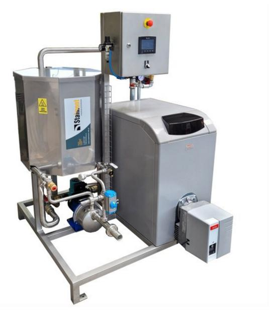
The pasteurizer is designed for thermal processing of fruit juices and purees - the previously squeezed juice is fed to a buffer tank, from where it is transported to a tubular exchanger where pasteurization takes place.
