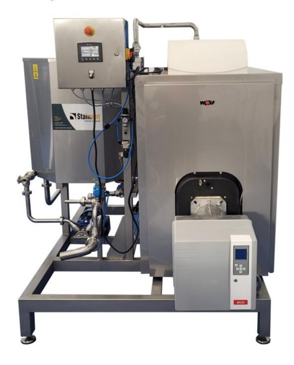
The pasteurizer is designed for thermal processing of fruit juices and purees - the previously squeezed juice is fed to a buffer tank, from where it is transported to a tubular exchanger where pasteurization takes place.
