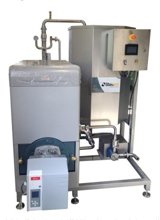
The pasteurizer is designed for thermal processing of fruit juices and purees - the previously squeezed juice is fed to a buffer tank, from where it is transported to a tubular exchanger where pasteurization takes place.
