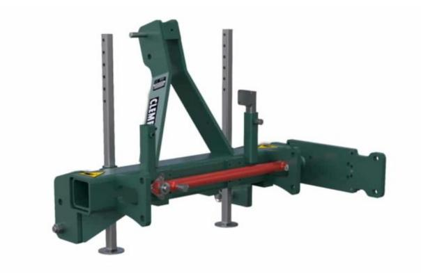
Would you like to work permanently with only a single-sided undervine care device, but as comfortably and safely as possible? For this case we have developed the SB MONO, which can be used for front and rear mounting. The hydraulic width adjustment can be easily converted from right to left. The base frame can be hydraulically adjusted by 500 mm from 960 to 1,460 mm on one side by means of a cylinder, either to the right or to the left.
