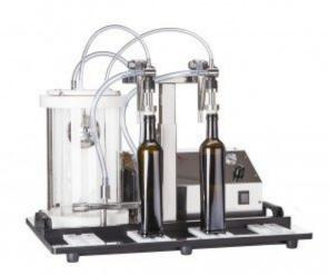
Enolmaster is a vacuum filler with small dimensions, very easy to use and at the same time filling the features of a very professional devices. The capacity of the device is up to 300 bottles (750 ml) per hour.
