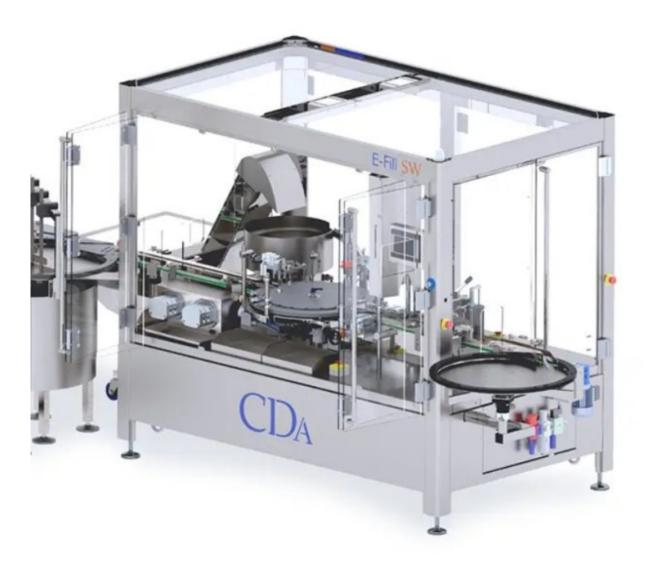
Automatic monoblock for filling, capping and labelling. The E-Fill SW Monoblock by CDA has been designed to ensure maximum efficiency and versatility in a fully automatic bottling line.
