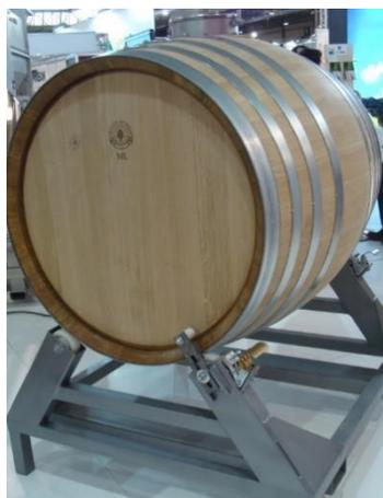
The rotative micro fermenter enables a gentle stirring thanks to the rotation (without crushing grapes skins and seeds).
